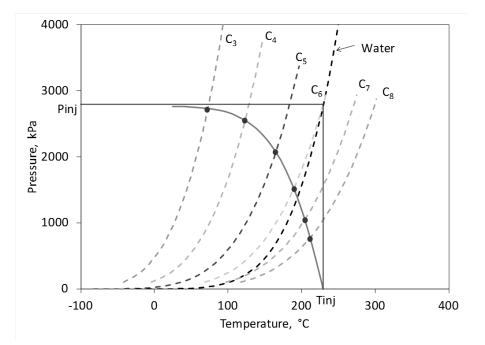
Figure 3-1. Example for solutions of Equation 3-2 for a few different single-component solvents at an injection pressure  $P_{inj}$ .
