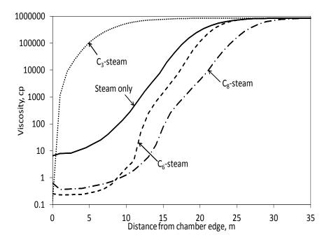
Figure 3-10. Profiles of the L phase viscosities in the 12<sup>th</sup> row of the reservoir model at 1.5 years.
