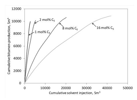
Figure 3-13. The cumulative oil production with respect to the cumulative volume of C<sub>5</sub> coinjected with steam.
