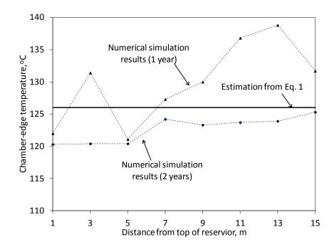
Figure 3-5. Comparison of numerical simulation results and estimations from Equation 3-2 for the chamber-edge temperature
