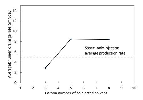
Figure 4-14. Results of numerical simulations of the base case for the average bitumen production rate after the 9th month of coinjection until the 20th month for 3 solvent-steam coinjection processes.
