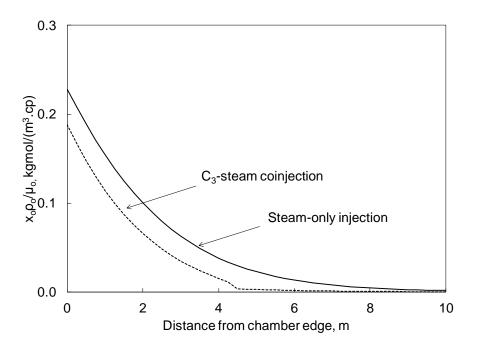
Figure 4-7. Profiles of the oil component molar flux integrand in Equation 4-14 vs. the perpendicular distance from the chamber interface for an assumed value of  $x_s^{edge} = 0.25$ .
