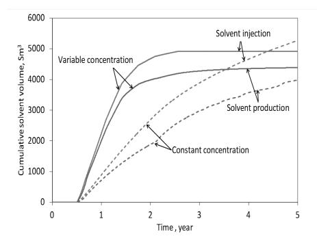
Figure 3-15. Injection and production volumes of  $C_5$  in coinjection simulations using two different injection procedures.
