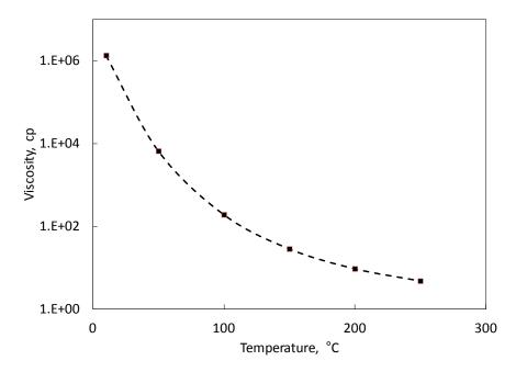
Figure 2-2. Viscosity of bitumen (the C<sub>D</sub> component in Table 2-2) at different temperatures.
