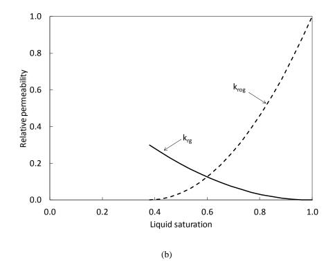
Figure 4-13. Relative permeability curves used in the simulation cases
