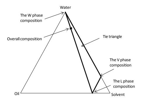
Figure 4-2. Tie triangle for a system of water, single component solvent and reservoir oil at a sample pressure and temperature.
