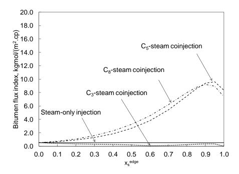
Figure 4-6. Profiles of the oil component drainageflux index in Equation 4-14 vs. the molar concentration of solvent in the L phase right at the chamber interface.
