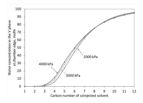
Figure 3-3. Water mole fraction in the V phase at the chamber edge edge for coinjection of a single-component solvent and steam.
