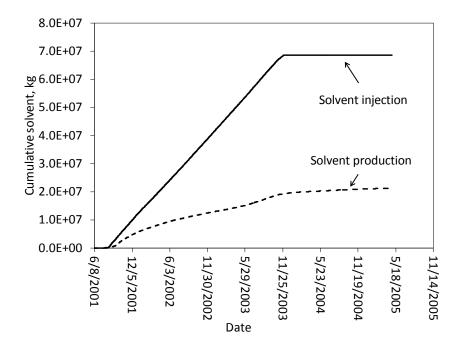
Figure 3-21. Cumulative solvent injection and production during SAP with scenario 2.
