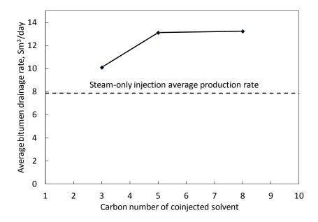
Figure 4-15. Results of numerical simulations of case 2 for the average bitumen production rate after the 5<sup>th</sup> month of coinjection until the 15<sup>th</sup> month for 3 solvent-steam coinjection processes.
