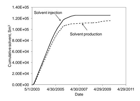
Figure 3-25. Injection and production volumes of C<sub>5</sub> for scenario 2 for the Long Lake ES-SAGD simulation.
