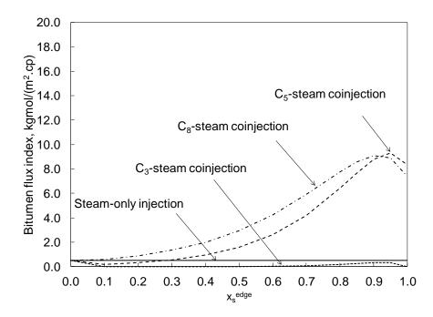
Figure 4-10. Profiles of the oil component drainage flux index in Equation 4-14 vs. the molar concentration of solvent in the L phase right at the chamber interface.
