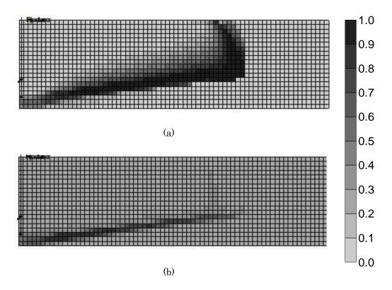
Figure 2-6. Gravity segregation of condensed water and solvent banks at 27 months in the ES-SAGD simulation.
