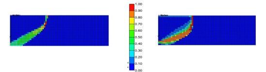
(b) Profiles of the  $C_5$  mole fraction in the L phase for  $C_5$ -steam coinjection at 1 year; Left:  $C_5$  concentration of 1 mol%, Right:  $C_5$  concentration of 8 mol%. The higher  $C_5$  concentration gives a thicker region of solvent accumulation near the chamber edge.
