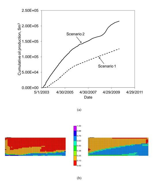
Figure 3-24. Comparison between Nexen's original process (scenario 1) and the modified coinjection (scenario 2) for the Long Lake ES-SAGD pilot.
