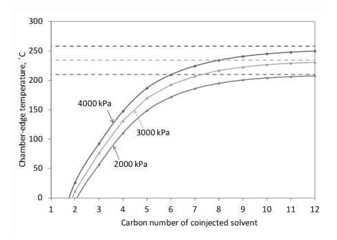
Figure 3-2. Chamber-edge temperatures estimation using Equation 3-2 for singlecomponent solvents from  $C_1$  to  $C_{12}$  for injection pressures of 2.0 MPa, 3.0 MPa, and 4.0 MPa.
