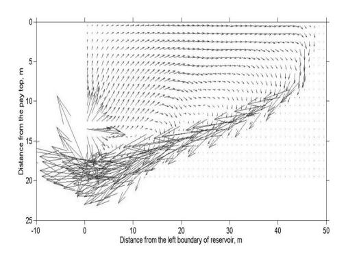
(a)  $C_4$  and steam coinjection, 23 months from the start of simulation.
