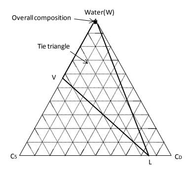
(e) 2 years from the start of the three-component ES-SAGD simulation. Gridblock (47, 7) is inside the ES-SAGD chamber. The V and L phases become less rich in  $C_5$ .
