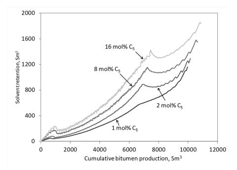
Figure 3-14. Solvent volumes retained in the reservoir for C<sub>5</sub>-steam coinjection simulations with different solvent concentrations.
