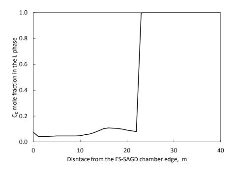
Figure 2-9. The C<sub>D</sub> mole fraction in the L phase at different distances from the chamber edge in the 14<sup>th</sup> row at 27 months in the ES-SAGD simulation.
