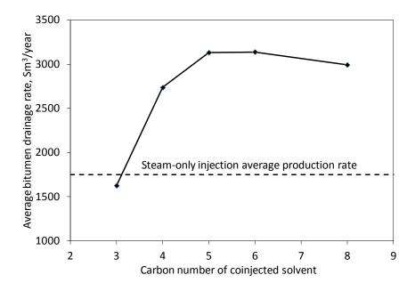
Figure 3-9. Average bitumen production rates for the first 2.5 years in Figure 3-8
