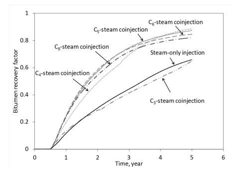
Figure 3-8. Oil recoveries for the steam-only injection and coinjection cases.
