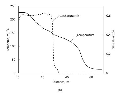
Figure 2-7. Distribution of the V phase saturation and temperature the 14<sup>th</sup> row at 27 months
