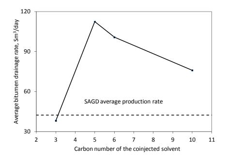
Figure 3-23. Average oil production rates for 1.5 years of the Long Lake ES-SAGD with different single-component solvents.
