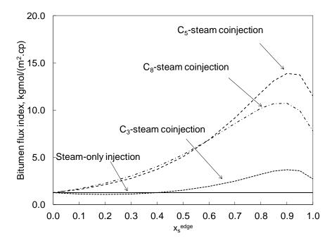
Figure 4-12. Profiles of the numerically evaluated oil component drainage flux index in Equation 4-14 vs. the molar concentration of solvent in the L phase right at the chamber interface.
