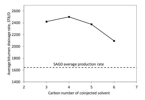
Figure 3-19. The average oil production rates after 8 months of SAP in simulations with different single-component solvents.
