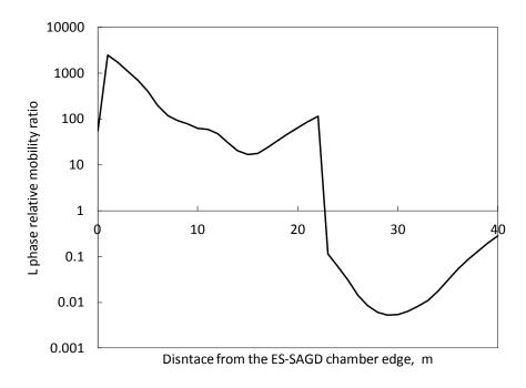
Figure 2-13. Relative mobility ratio at different distances from the chamber edge in the 14<sup>th</sup> row at 27 months.
