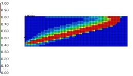
(d) Profiles of the  $C_5$  mole fraction in the L phase for  $C_5$ -steam coinjection at 2 years; Left:  $C_5$  concentration of 1 mol%, Right:  $C_5$  concentration of 8 mol%. Continuous coinjection of a high-concentration solvent results in an unfavorably thick region of solvent accumulation. This can lead to a significant amount of solvent being trapped near the chamber edge by the end of process.
