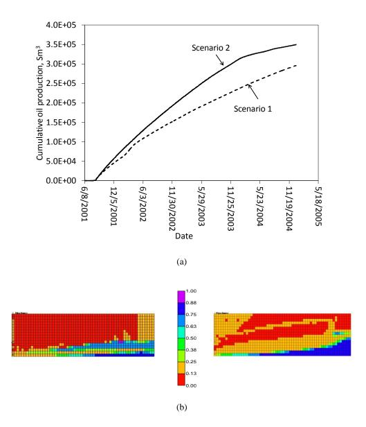
Figure 3-20. Comparison of EnCana's original operation (scenario 1) and a modified coinjection process (scenario 2) for the Senlac SAP pilot.
