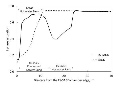
Figure 2-10. Distribution of the L phase saturation at different distances from the chamber edge in the 14<sup>th</sup> row at 27 months in the ES-SAGD and SAGD simulations.
