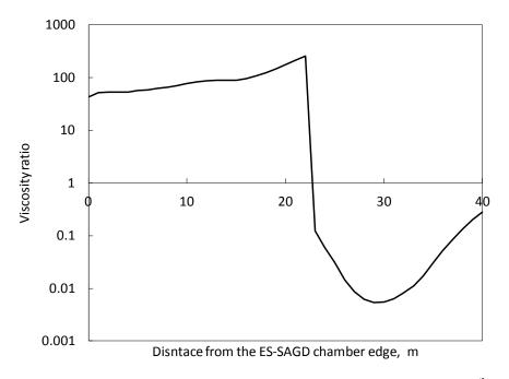
Figure 2-12. Viscosity ratio at different distances from the chamber edge in the 14<sup>th</sup> row at 27 months.
