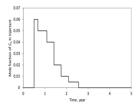
Figure 3-16. Variation of the solvent concentration in the injectant during the modified coinjection procedure.
