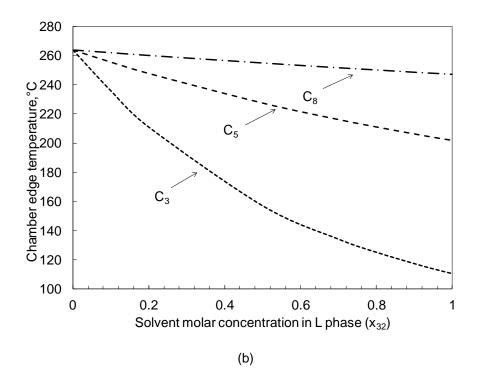
Figure 4-3. Variations of chamber edge temperature vs. solvent mole fraction in the L phase  $(x_{32}=z_3/(z_3+z_2))$
