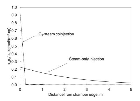
Figure 4-8. Profiles of the oil component molar flux integrand in Equation 4-14 vs. the perpendicular distance from the chamber interface for an assumed value of  $x_s^{edge} = 0.7$ .
