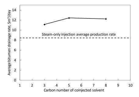
Figure 4-16. Results of numerical simulations of case 3 for the average bitumen production rate after the 4<sup>th</sup> month of coinjection until the 15<sup>th</sup> month for 3 solvent-steam coinjection processes.
