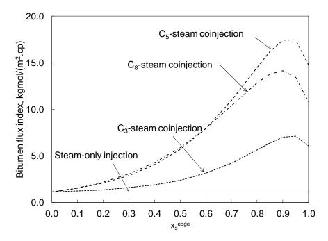
Figure 4-11. Profiles of the numerically evaluated oil component drainage flux index in Equation 4-14 vs. the molar concentration of solvent in the L phase right at the chamber interface.
