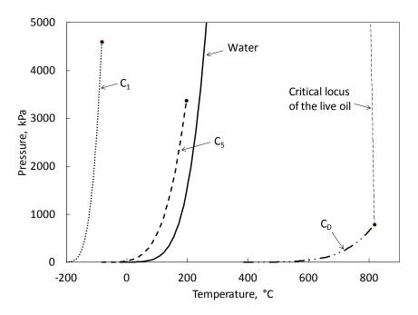
Figure 2-3. Vapor pressure curves of  $C_1$ ,  $C_5$ ,  $C_D$ , and water, and the critical locus of the live oil (a mixture of  $C_1$  4% and  $C_D$  96%).
