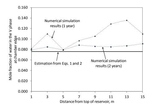
Figure 3-6. Comparison of numerical simulation results and estimations from Equation 3-1 for the water mole fraction in the V phase at the chamber edge.
