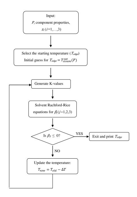
Figure 4-1. Flowchart of the algorithm used for estimation of  $T_{edge}$  for a given pressure and an assumed overall composition.
