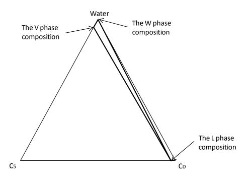
Figure 2-5. Tie triangle for the water,  $C_5$ , and  $C_D$  mixtures at 224.5°C and 2715 kPa (conditions inside the chamber).
