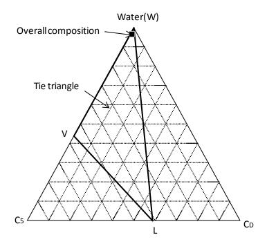
(d) 18 months from the start of the three-component ES-SAGD simulation. Gridblock (47, 7) is just inside the ES-SAGD chamber. The L phase in the previous figure is split into the V and L phases in the presence of the invariant W phase.
