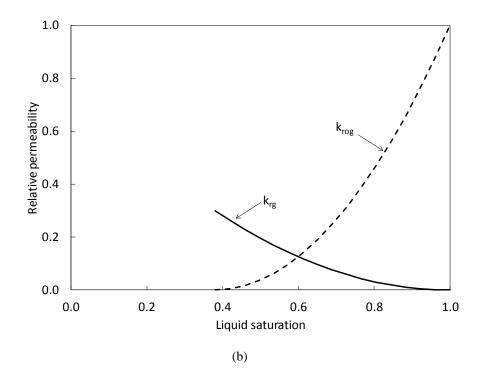
Figure 2-1. Relative permeability curves used in the simulation cases.
