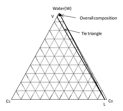
(d) 18 months from the start of the three-component ES-SAGD simulation. The  $C_D$  concentration in the tie triangle is not as small as in gridblock (47, 7) given in Figure 2-17, resulting in a higher L phase mole fraction.
