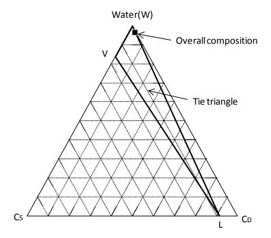
(c) 4 months from the start of the three-component ES-SAGD simulation. The  $C_D$  concentration in the tie triangle is not as small as in gridblock (47, 7) given in Figure 2-17, resulting in a higher L phase mole fraction.
