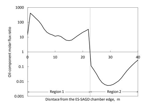
Figure 2-15. Oil-component molar flux ratio at different distances from the chamber edge in the 14<sup>th</sup> row at 27 months.
