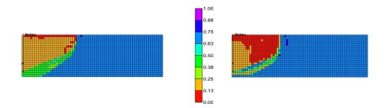
(a) Profiles of the L phase saturation in C<sub>5</sub>-steam coinjection at 1 year; Left: C<sub>5</sub> concentration of 1 mol%, Right: C<sub>5</sub> concentration of 8 mol%. Regions in red indicate enhanced local displacement efficiency with the L phase saturations below  $S_{or}$ . The higher C<sub>5</sub> concentration gives higher local displacement efficiency.
