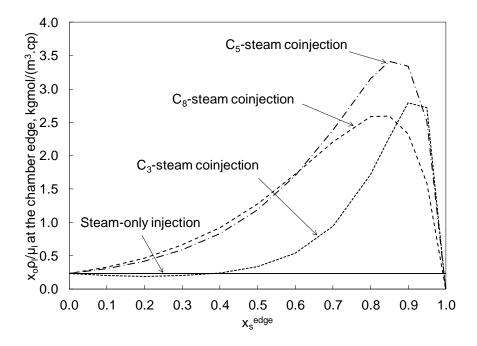
4-5. Variations of the oil component molar flux integrand in Equation 4-14 vs. the molar concentration of solvent in the L phase right at the chamber interface.
